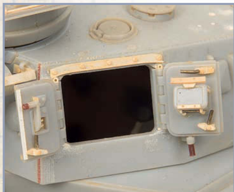
The open hatches were reworked by removing and replacing the moulded on locking handles and adding the rubber cushions to the vision block.
