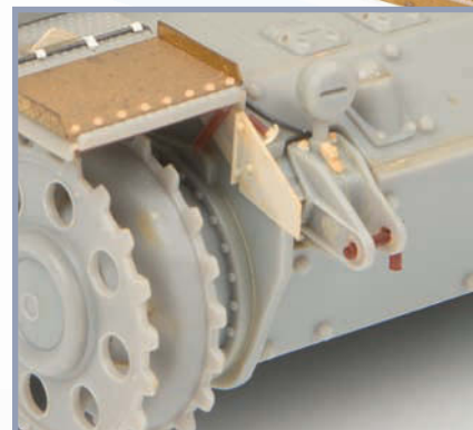
The front mudflap arrangement and the towing hooks required quite a lot of additional detail work with the missing side panels added and the latch clips for the mudflap.
