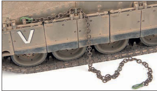
The tow chain supplied in the kit was treated in the blackening solution and the shackles were finished in green.
